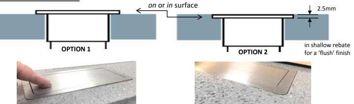
In either of these "surface-mount" methods, it is also possible to 'personalise' the unit, by **replacing** the standard stainless steel top with a piece of matching material to the work top if required.
