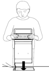
Surface Mounted (flush) As above but set in into a shallow 2.5mm rebate for a 'flush' finish.
