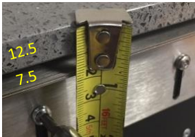
The S-Box mounting collar is adjustable to accommodate up to 1/2" (12.5mm) custom top material.
