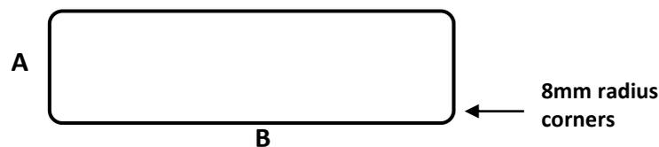
Then create a **further** 8mm wide rebate **at 20mm depth** from the top of the work-surface, on which to mount the S-Box, and its collar, in its new position. The radius of the collar's corners is 8mm, so we suggest that you use a maximum 10mm radius for the rebate-routing process.
