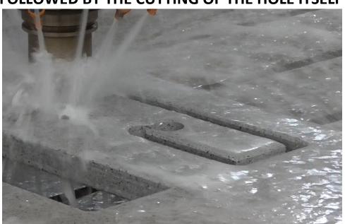
THE TOOL THEN RETURNS TO THE WORKTOP TO CARRY OUT ITS SECOND GRINDING PROCESS AND CREATES THE REBATE (at -20mm DEPTH) FOR THE S-BOX™ COLLAR TO SIT ON LATER.
