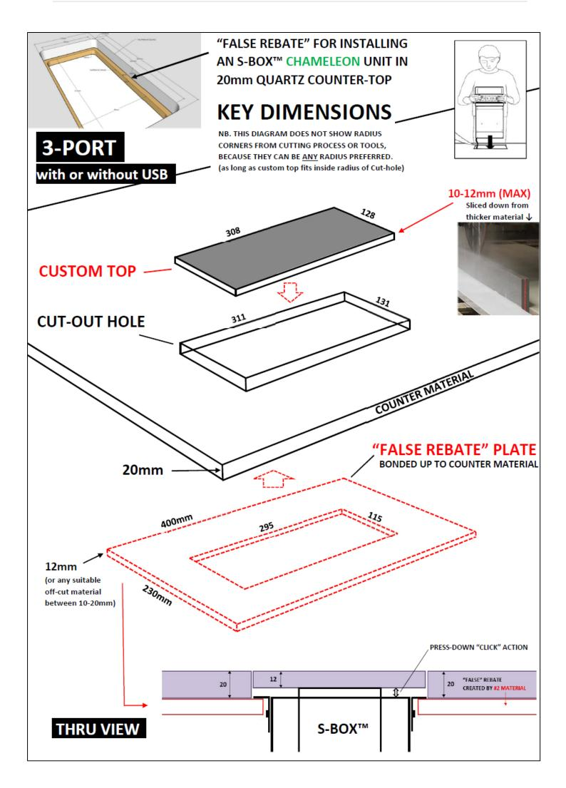
IF TOP MATERIAL IS 12mm THICKNESS, THE SLAVE MATERIAL SHOULD BE 18-20mm AND REQUIRES ITS OWN SHALLOW REBATE TO CREATE A TOTAL REBATE OF 20mm.
