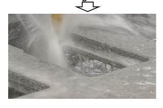
TO CREATE THE REBATE IN 30mm MATERIAL – THE ROUTER CARRIES OUT <u>TWO</u> PROCESSES: THE FIRST IS A FULL THRU-CUT HOLE. THE SECOND IS TO GRIND OUT AN EXTRA 8mm, AT 20mm DEPTH.
