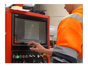
THE CUTTING TOOLS (TYPICALLY CROSS-CUTTER and CNC ROUTER) ARE PROGRAMMED WITH THE DIMENSIONS REQUIRED.
