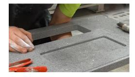
WITH HOLES AND TOPS NOW READY, THE COUNTERTOP CAN GO TO SITE . . . FOR THE S-BOX™ UNIT TO BE INSTALLED! ☺
