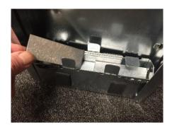
ADDITIONAL COUNTERWEIGHTS HAVE BEEN PROVIDED, SO THAT THE PARTICULAR DENSITY OF ANY 12mm "CUSTOM TOP" MATERIAL CAN BE OFFSET TO MAINTAIN THE UNIT'S SELF-LIFT.
