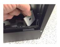
Take the New Top off and introduce the S-Box unit into its rebated hole.
