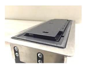
This re-creates the clearance required below the *later* new top - so that when it is pressed down it will engage and disengage the catch mechanism inside the unit. Re-tighten the collar screws (with the new top temporarily  $\downarrow$  in position) so that the required 20mm total is achieved (as below)
