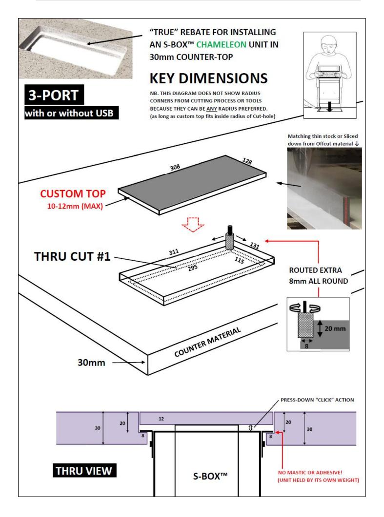
CREATING THE REBATE WITH 20mm MATERIAL REQUIRES THE USE OF A SECOND/'SLAVE" PLATE. THE DIFFERENCE BETWEEN THE UPPER HOLE DIMS, AND THOSE OF THE SLAVE, <u>CREATES</u> THE REBATE. CUSTOM TOP DIMENSIONS ARE 3mm SMALLER, TO PRODUCE A 1.5MM GAP TO ALL 4 SIDES.
