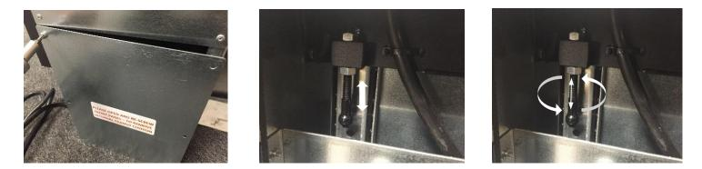
**REMINDER:** THE COMPLETED UNIT SHOULD NOT BE PERMANENTLY FIXED INTO ITS REBATE. ITS OWN WEIGHT WILL KEEP IT IN POSITION. THIS ENSURES THAT IN THE EVENT THAT THE UNIT NEEDS TO BE EXTRACTED FOR ANY REASON IT CAN BE LIFTED OUT THROUGHT THE SURFACE
