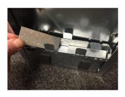
ADDITIONAL COUNTERWEIGHTS HAVE BEEN PROVIDED, SO THAT THE PARTICULAR DENSITY OF ANY 12mm "CUSTOM TOP" MATERIAL CAN BE OFFSET TO MAINTAIN THE UNIT'S SELF-LIFT.
