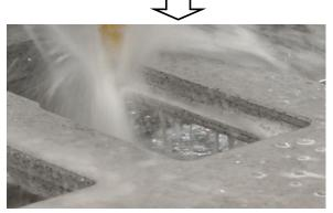
TO CREATE THE REBATE IN 30mm MATERIAL – THE ROUTER CARRIES OUT <u>*TWO*</u> PROCESSES: THE FIRST IS A FULL THRU-CUT HOLE. THE SECOND IS TO GRIND OUT AN EXTRA 8mm, AT 20mm DEPTH.
