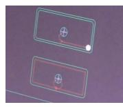
NB. A ROUTER STARTS ITS CUTTING ROUTE FROM THE <u>CENTRE POINT</u> WHEN IT MACHINES OUT ANY HOLE.
