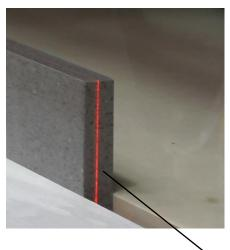
THE 12mm (<u>maximum</u>) S-BOX<sup>™</sup> CUSTOM TOP IS MADE BY 'SLICING' AN OFF-CUT PIECE OF THE COUNTER MATERIAL . . . . <u>OR</u> CAN BE MADE FROM 12mm MATCHING STOCK.
