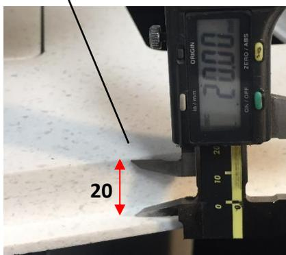
THE S-BOX™ COLLAR IS ADJUSTABLE TO ENSURE THAT THE UNIT (AND ITS TOP) FIT INTO THE 20mm REBATE
