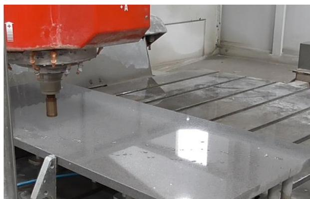
**In 20mm material (or less) the hole will only be a full thru-cut one, with the rebate added later by using a second material underneath)**
