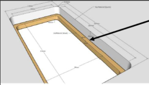
"FALSE REBATE" FOR INSTALLING AN S-BOX™ CHAMELEON UNIT IN 20mm QUARTZ COUNTER-TOP.
