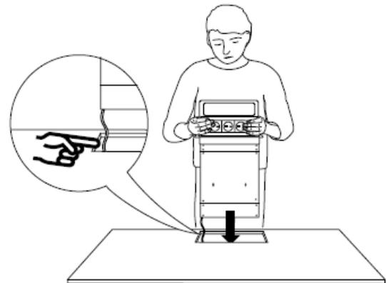
↑ The black collar is perfectly OK on its own, and is deliberately designed to suit nil or very tight radius corners from the cutting process
