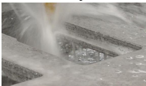
TO CREATE THE REBATE IN 30mm MATERIAL – THE ROUTER CARRIES OUT TWO PROCESSES: THE FIRST IS A FULL THRU-CUT HOLE. THE SECOND IS TO GRIND OUT AN EXTRA 8mm, AT 20mm DEPTH. THE CUSTOM TOP DIMENSIONS ARE 3mm SMALLER, TO PRODUCE A 1.5MM GAP TO ALL 4 SIDES. (see 'custom top' process on page 10)
