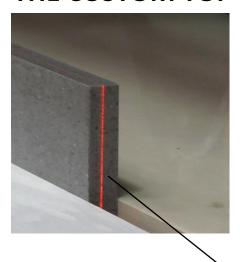
THE 12mm (maximum) S-BOX™ CUSTOM TOP IS MADE BY 'SLICING' AN OFF-CUT PIECE OF THE COUNTER MATERIAL . . . . OR CAN BE MADE FROM 12mm MATCHING STOCK.
