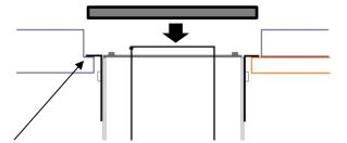
\* DO NOT USE ANY MASTIC OR ADHESIVE HERE. UNIT <u>MUST</u> BE REMOVEABLE IF REQUIRED. IT USES ITS OWN WEIGHT FOR STABILITY. FOR STONE (GRANITE and QUARTZ) MATERIAL PLEASE ADD 3-4 OF SPOTS OF MASTIC FOR EXTRA ADHESION
