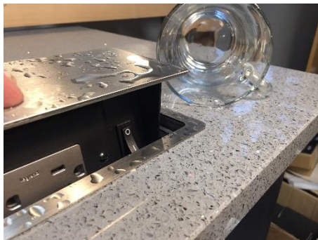
UL962A + NEC 2 litre (½ Gallon) Saline Liquid Test 406.5 (E)
