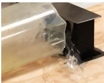
UL962A + NEC 2 litre (½ Gallon) Saline Liquid Test 406.5 (E)
