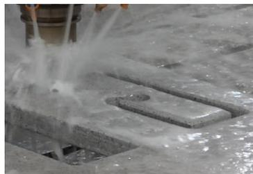
Router-tool cutting the hole
