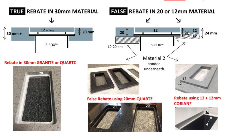
SO ANY S-BOX™ THAT IS TO BE INSTALLED IN THE HIDDEN "CHAMELEON" MODE, NEEDS THE INVOLVEMENT OF THE WORKTOP FABRICATOR AND HIS CUTTING TOOLS . . .
