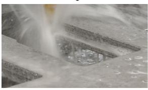
TO CREATE THE REBATE IN 30mm MATERIAL – THE ROUTER CARRIES OUT <u>TWO</u> PROCESSES: THE FIRST IS A FULL THRU-CUT HOLE. THE SECOND IS TO GRIND OUT AN EXTRA 8mm, AT 20mm DEPTH.
