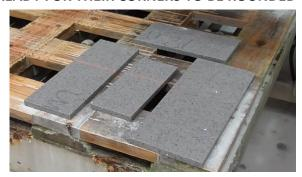
THE CORNERS ARE TYPICALLY ROUNDED BY HAND TO ENSURE THAT THE CUSTOM TOPS WILL NEATLY MARRY WITH THE INTERNAL RADIUS OF THE HOLES. THE EXPERIENCE AND SKILL OF THE WORKTOP SUPPLIER ENSURES THAT EVERYTHING WILL FIT BEAUTIFULLY ON SITE.
