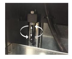
THE COMPLETED UNIT SHOULD NOT BE PERMANENTLY FIXED INTO ITS REBATE. ITS OWN WEIGHT WILL KEEP IT IN POSITION. THIS ENSURES THAT IN THE EVENT THAT THE UNIT NEEDS TO BE EXTRACTED FOR ANY REASON IT CAN BE LIFTED OUT THROUGHT THE SURFACE
