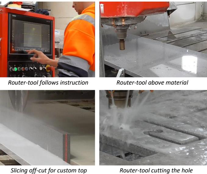
This rebate is either a **"True"** - one that is pre-cut by a router **within thick material (30mm and over)**
