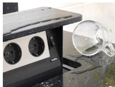
NEC 2.2 litre (½ Gallon) Saline Liquid Spill Test 406.5 (E)
