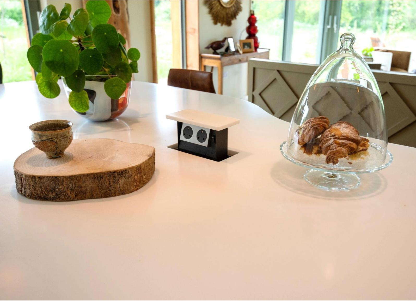
**S-BOX™ CHAMELEON MODELS** are supplied with a special 'any-radius' black collar. This is pre-set and fixed for installation of the unit **at -20mm below the surface on a rebate shelf** – one that is pre-cut within (or 'created' below) the counter material. The unit is therefore ready to receive a piece of worktop material **up to 12mm thick maximum** – to be used as the unit's top.
