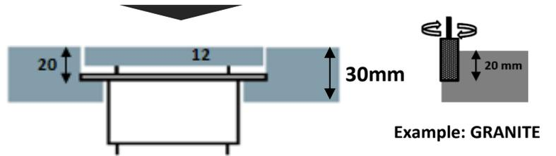
**OR** it is a **"False"** rebate. This is one that is *created* directly below thinner material (20mm or less) by using a **secondary material bonded underneath** to 'create' the shelf.
