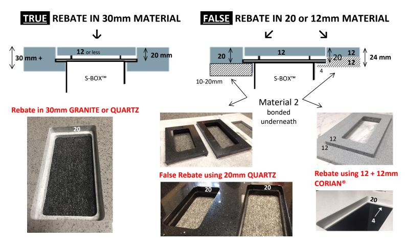
SO ANY S-BOX<sup>™</sup> THAT IS TO BE INSTALLED IN THE HIDDEN "CHAMELEON" MODE, NEEDS THE INVOLVEMENT OF THE WORKTOP FABRICATOR AND HIS CUTTING TOOLS . . .
