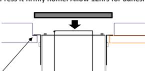
\* DO NOT USE ANY MASTIC OR ADHESIVE HERE. UNIT <u>MUST</u> BE REMOVEABLE IF REQUIRED. IT USES ITS OWN WEIGHT FOR STABILITY.
