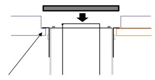
\* DO NOT USE ANY MASTIC OR ADHESIVE HERE. UNIT <u>MUST</u> BE REMOVEABLE IF REQUIRED. IT USES ITS OWN WEIGHT FOR STABILITY.
