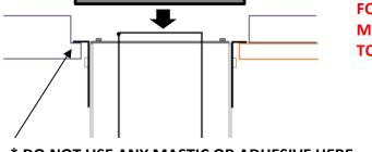
\* DO NOT USE ANY MASTIC OR ADHESIVE HERE. UNIT <u>MUST</u> BE REMOVEABLE IF REQUIRED. IT USES ITS OWN WEIGHT FOR STABILITY.
