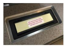
For lightweight materials that are dry and free from dust, (like Timber or Corian) peel back the tape and place the custom top into position. Press it firmly home. Allow 12hrs for adhesive to bond and cure.
