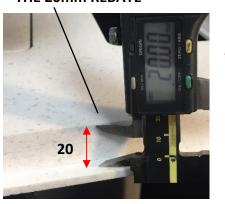
THE COLLAR IS ADJUSTABLE TO ENSURE THAT THE UNIT <u>AND ITS TOP</u> ARE "4-SIDE PARALLEL" & FIT INTO THE 20mm REBATE
