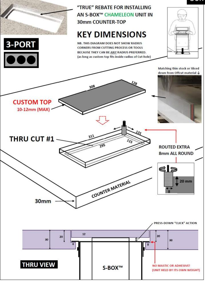
CREATING THE REBATE WITH 20mm MATERIAL REQUIRES THE USE OF A SECOND/'SLAVE" PLATE. THE DIFFERENCE BETWEEN THE UPPER HOLE DIMS, AND THOSE OF THE SLAVE, CREATES THE REBATE.
